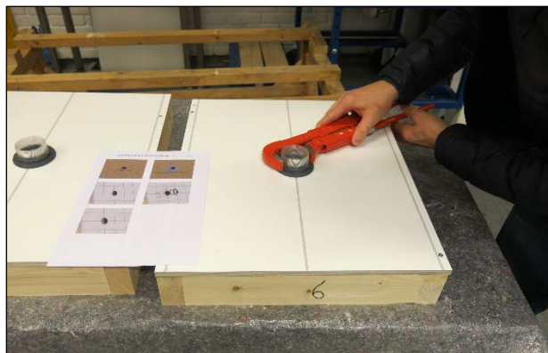
Fig. 5.1.2: Inserting and tightening of Roth Sealing Ring.
